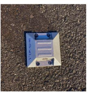
**Ground Monitoring Points** are passive, surface mounted devises used to survey the ground surface before, during, and after tunnel construction.
